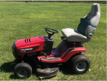
Murray 12.5 HP Lawn Mower with 40 inch Mower Deck, 4 spd. Trans., Luxury Seat
